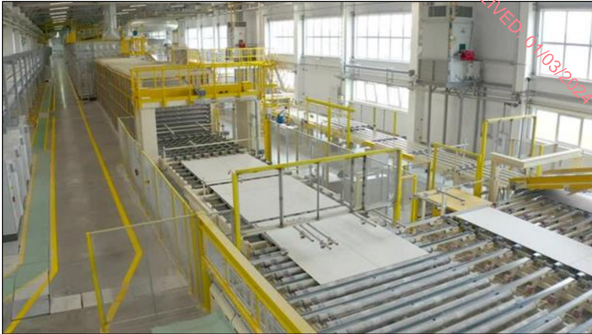
Figure 3-5: Plasterboard Entering a Dryer
